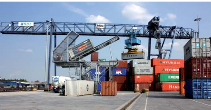
The new tipping platform at the Rhein-Ruhr Terminal speeds up the process of loading granulates into silos.
